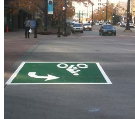
Figure 1: example of a two-stage turn box
