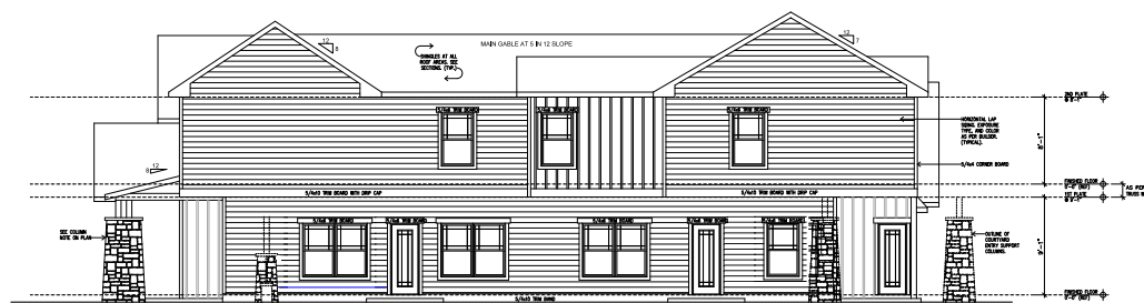
LEFT ELEVATION THE COURTYARD (COURTYARD SIDE) SCALE: 1/4" = 1'-0"
