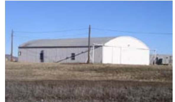
Figure 2. While similar in its roofline and exterior cladding to a true Quonset hut, this airplane hangar differs in that vertical walls comprise most of the side elevations. It is located at Christman Field, on CSU’s Foothills Campus. (Photo by the author)
