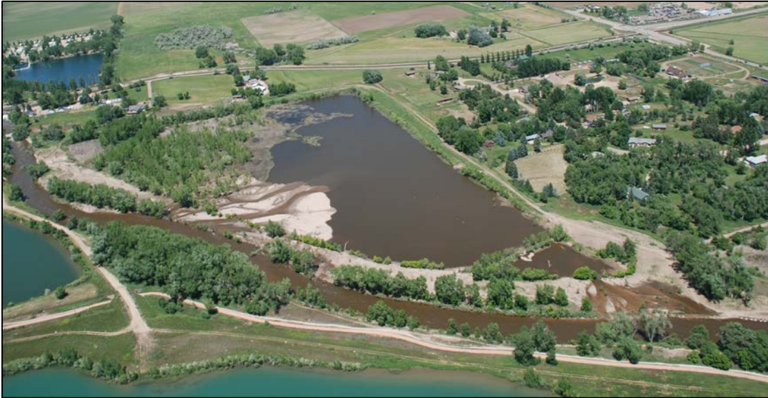
Figure IV.2 Recent lowering of a high berm (remnant from gravel mining activity) between the Poudre River and Sterling Pond upstream of Shields St. allowed high spring flows in June 2014 to overtop its banks, inundate a wider riparian area, and flow into the pond.
