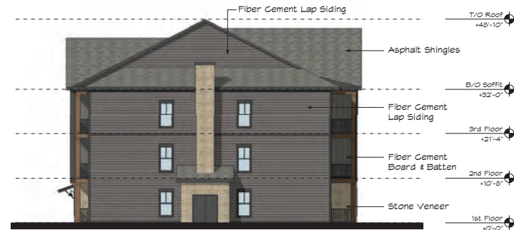
SIDE ELEVATION - BUILDING TYPE C
