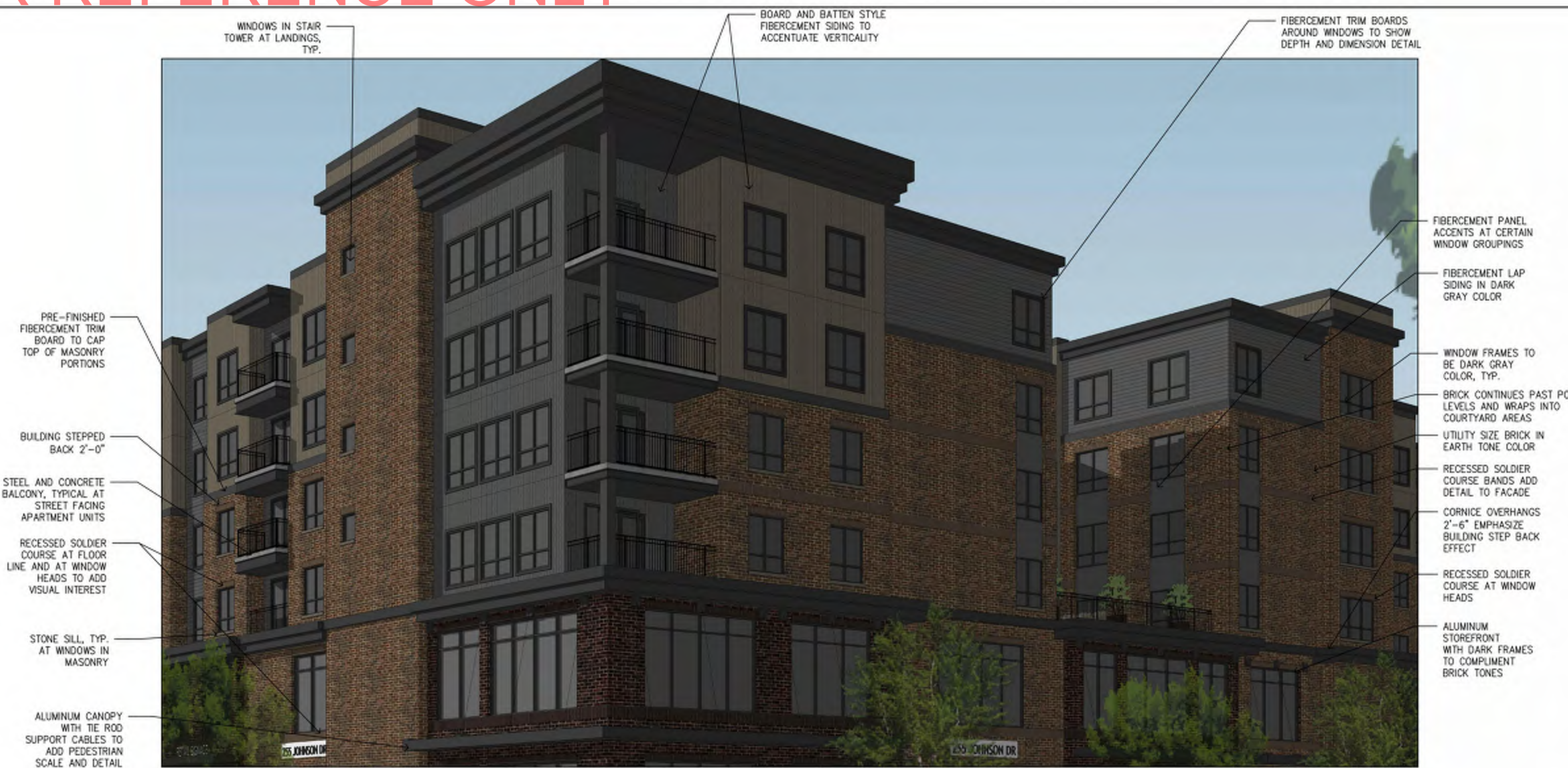
NORTHEAST ENTRY - MATERIAL DETAIL VIEW
