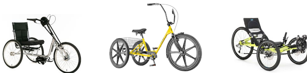
Figure 5. Trikes in the adaptive library fleet: hand trike (left), upright trike (middle), recumbent trike (right)
