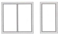
ALL INSTALLATIONS TO HAVE 4' to 6' WIDE X 4' to 6' TALLYINYL OR FIBERGLASS SLIDING WINDOW or 30" to 48" WIDE X 4' to 6' TALL CASEMENT WINDOW WITH U FACTOR LESS THAN 0.28
