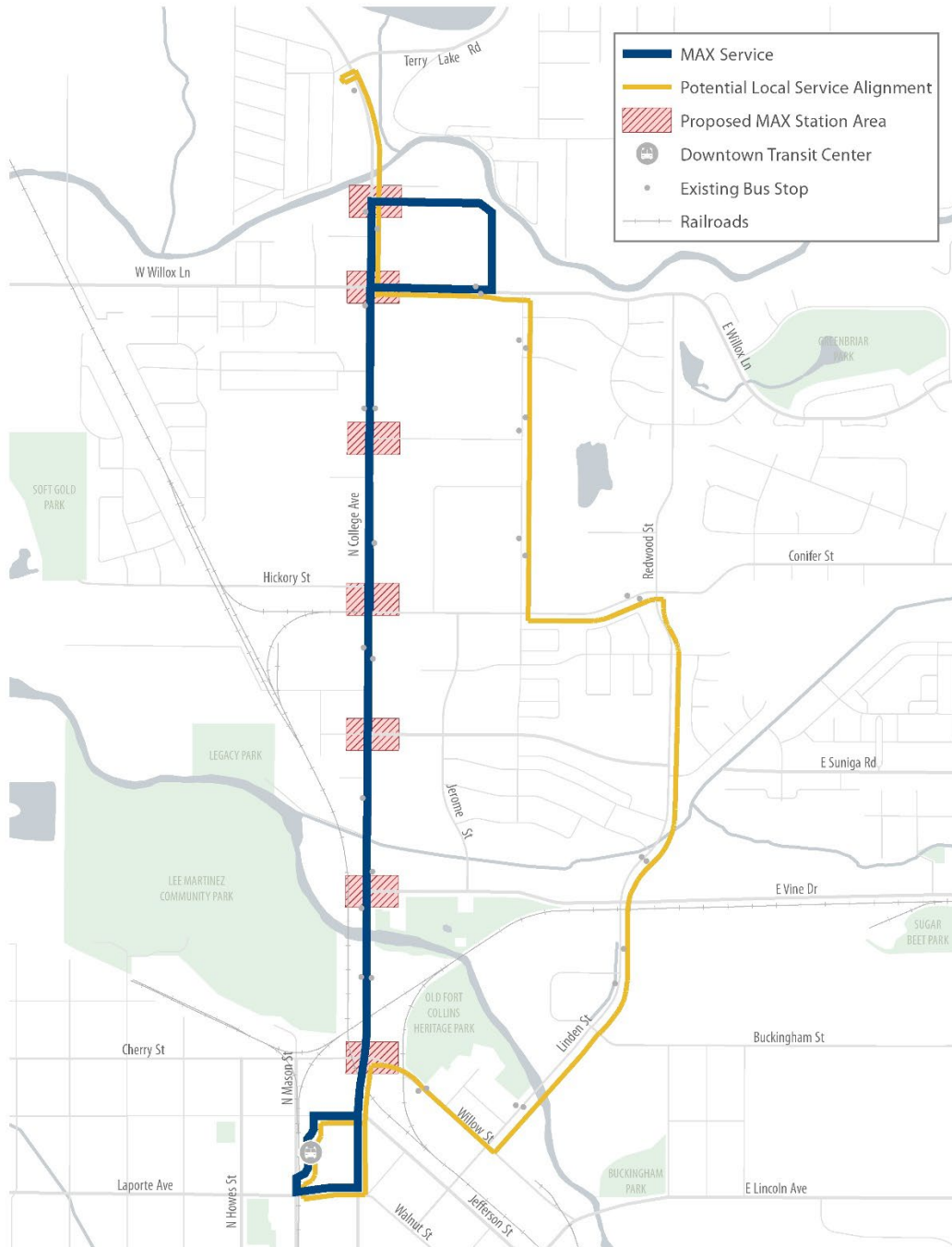
Figure 2: Map of Alternative 2 - MAX on North College with Turnaround on King Soopers Internal Roadway
